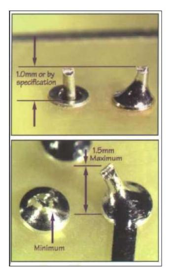
We strictly recommend in this case not to bend the pins during the length adjustment process as this will weaken them and may cause internal damage to the converter. Therefore a special leveling tool may be required for this operation, this could be as simple as a piece of aluminum plate cut to the same level of the pins length and drilled slightly larger than the pins diameter (0.3~0.5mm or 0.012~0.02").
